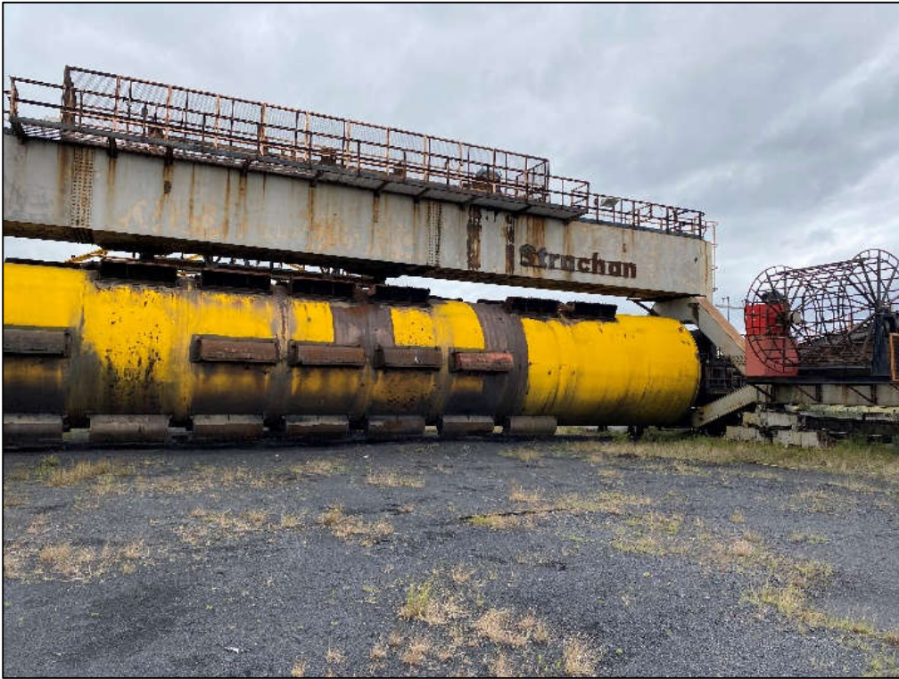
Photograph 5 - Area 10 Barrel Reclaimer
